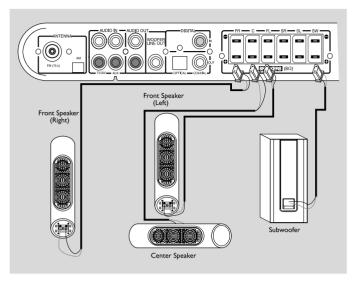
Connect the supplied speaker system using the supplied speaker cables by matching the colours of the jacks and speaker plugs. Fully insert the plugs of speaker wire into the jacks on the DVD system.
